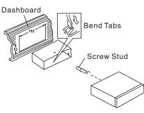
slides into the opening. Do not force the sleeve into the opening or cause it to bend or bow. Check that there will be sufficient space behind the dashboard for the radio chassis.
